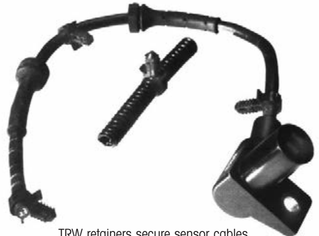
TRW retainers secure sensor cables
